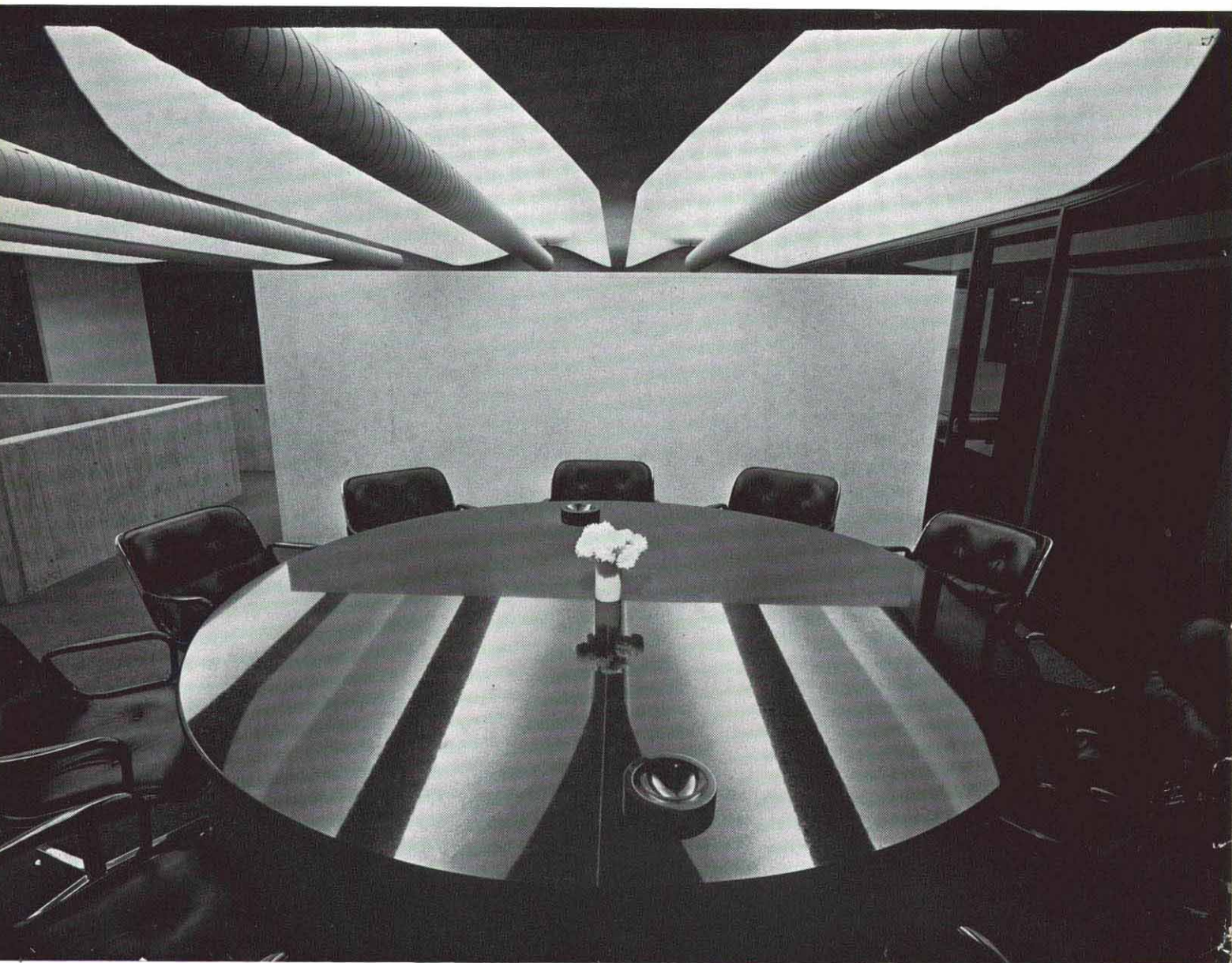
Milsons Point office interior, showing the integration of air-conditioning ducts, lighting and precast prestressed concrete floor units.
